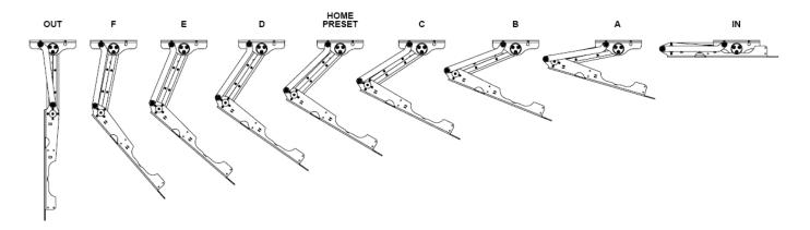
A number of preset positions are set in the mechanism which are shown above with the corresponding letter on the remote control.
